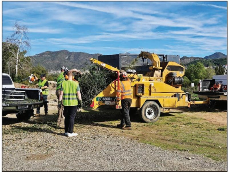
A heavy-duty chipping machine turns tree branches into wood chips.
