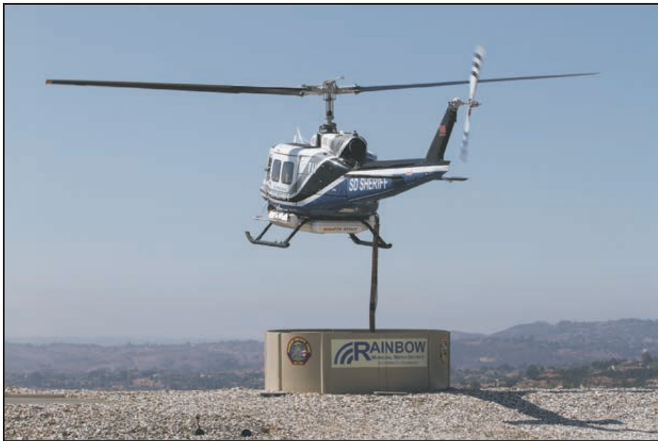
Water is pumped from the heli-hydrant during an unveiling in Fallbrook, Nov 9. The heli-hydrant and wind sock is LED illuminated to allow pilots to safely make refills at night during a firefight. Pilots are also able to wirelessly fill the tank at the push of a button.
