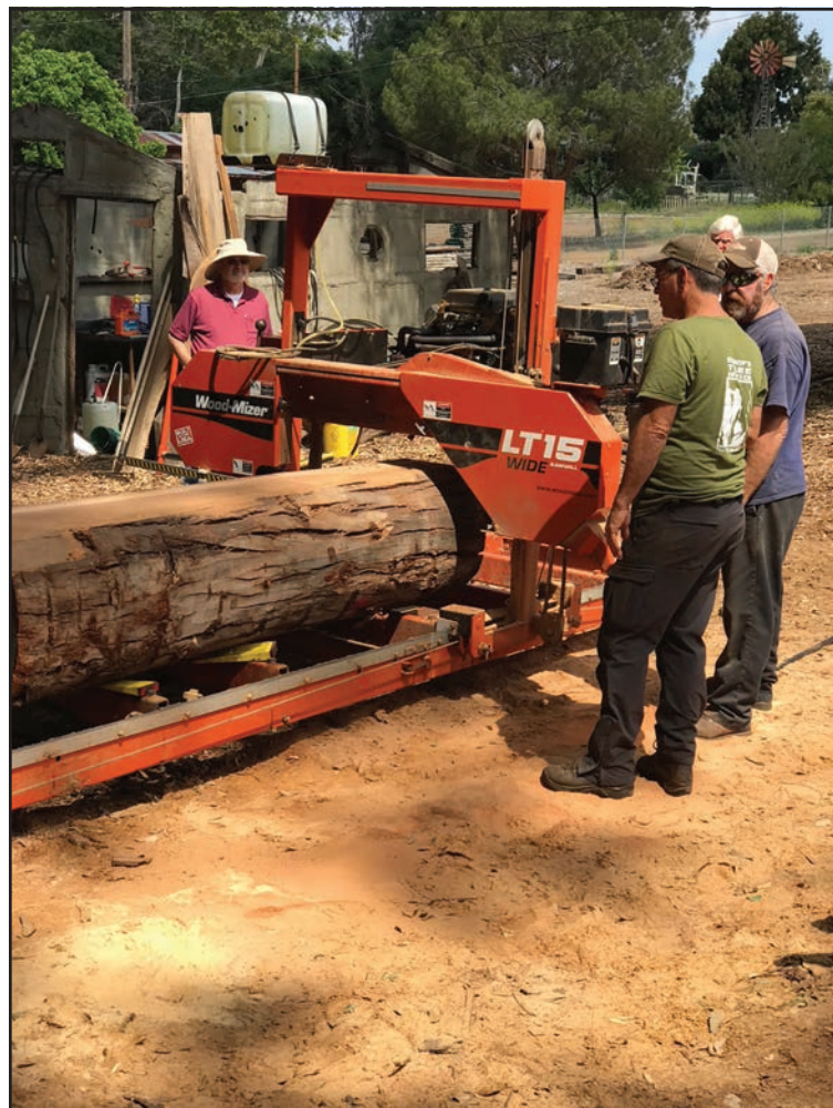
Brian Bishop, who is wearing a green shirt, is seen with his company's Wood Mizer portable sawmill which is cutting a log into planks, giving new life to old wood.
