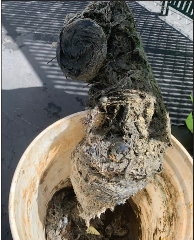
This is what a ball of wet wipes looks like when they all clump together at one of the lift stations. Village News/Rainbow Water photo by multiple items clogging together the problem might not be found immediately. “Sometimes they don’t show up right away,” Bebee said. “If people start to do it on a large scale, it will cause problems,” Bebee said. “It’s something that’s important to keep that under control.” Joe Naiman can be reached by email at jnaiman@reedermedia.com .
