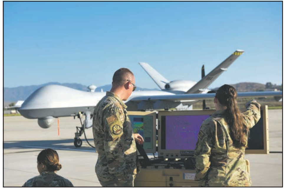
Airman 1st Class Anika Manabat, Staff Sgt. Jacob Allen and Airman 1st Class Jaiden Bainbridge from the 432nd Aircraft Maintenance Squadron operate a Portable Aircraft Control Station for an MQ-9 Reaper remotely piloted aircraft at Marine Base Camp Pendleton, Aug. 23. The MQ-9 Reaper was being prepped for its first launch from Marine Base Camp Pendleton.
