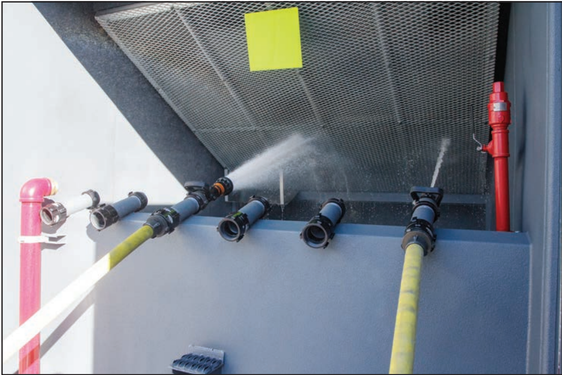
Water is shot from fire hoses affixed to one fire truck; the water is collected in the tank of the Pump Pod and then pumped into a second fire truck's tank which then pumps it back into the first fire engine's tank.
