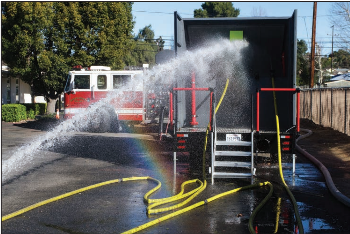
Firefighters can vary the amount of water pressure in the hoses as they spray up to 1250 gallons per minute into the 1800 gallon tank in the Pump Pod.
