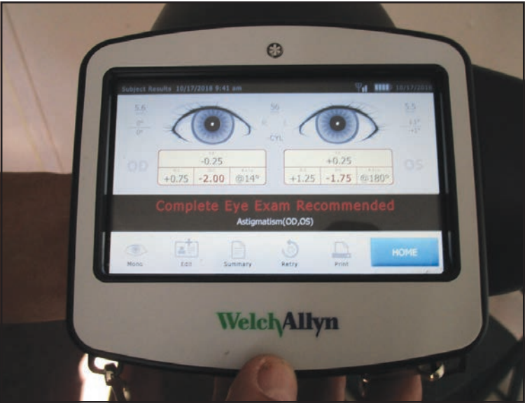
The Spot Vision Screener measures the physical condition of a person’s eyes and can identify problems like astigmatism.
