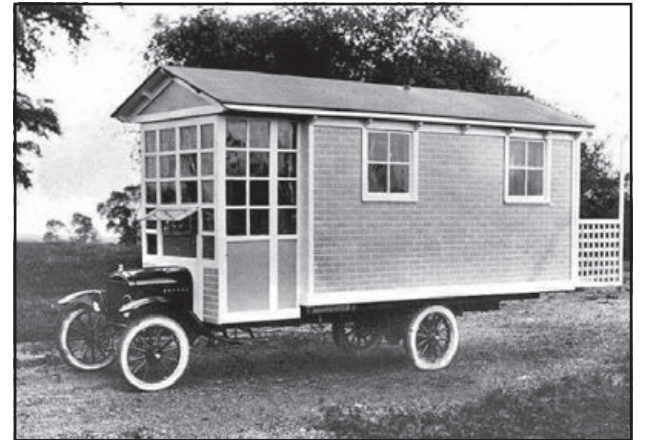
From the mid-teens and into the 1920s many small home-built motorhomes were constructed on the inexpensive Ford Model T car and Model TT truck chassis.
