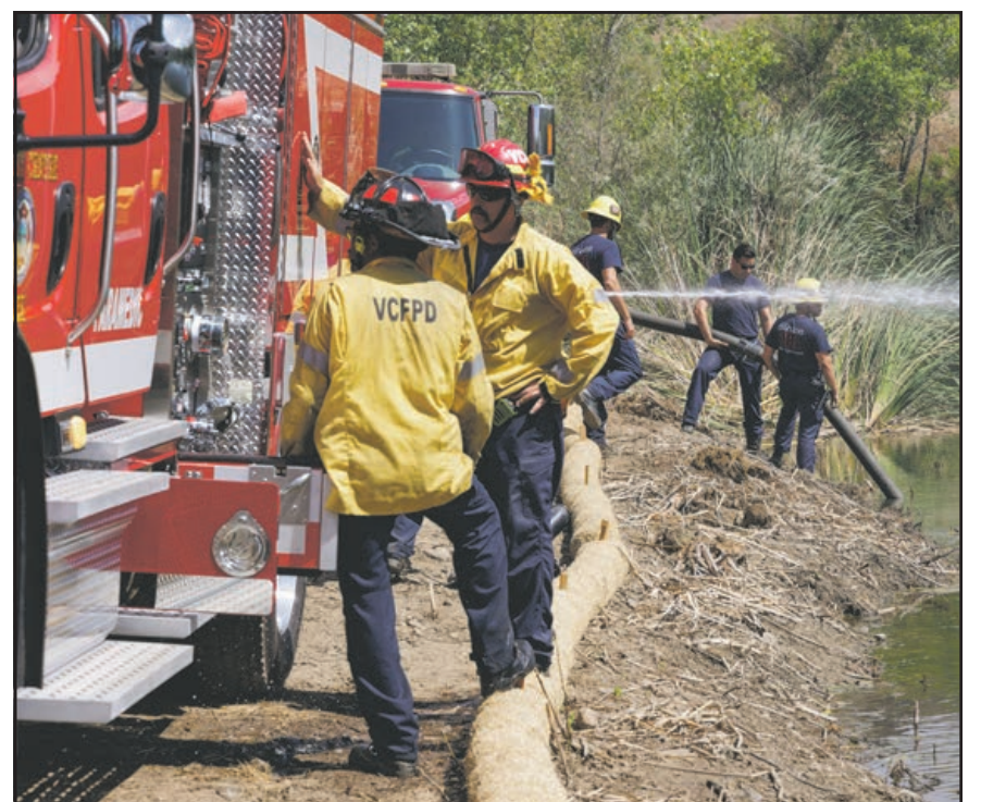
Firefighters practice pumping water from the Gomez Creek ponds and cycling the water through fire engine hydraulics and out their fire hoses during a pump-in event.
