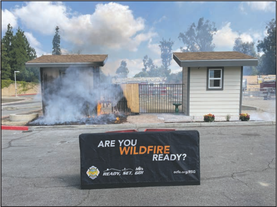
Two demonstration ‘houses’ sit side by side as small fires are lit near each one. The house on the left has plants near the structure, surrounded by wood chips and a wooden fence. While the fire on the right does not spread to the house, the fire on the left is burning the wood chips, plants, fence, and the house. Village News/ Kara Garrett photos
