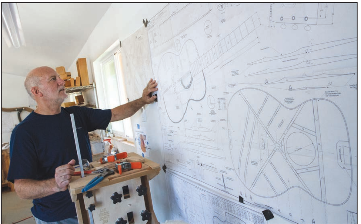
Luthier Shawn Weimer looks over blueprints of acoustic guitar designs invented by Christian Frederick Martin Sr. Martin revolutionized acoustic guitar design in the 1830s which included X-bracing. Martin's innovative flattop guitar design is still in use today by many guitar makers including the structural inspiration for Weimer's acoustic creations.
