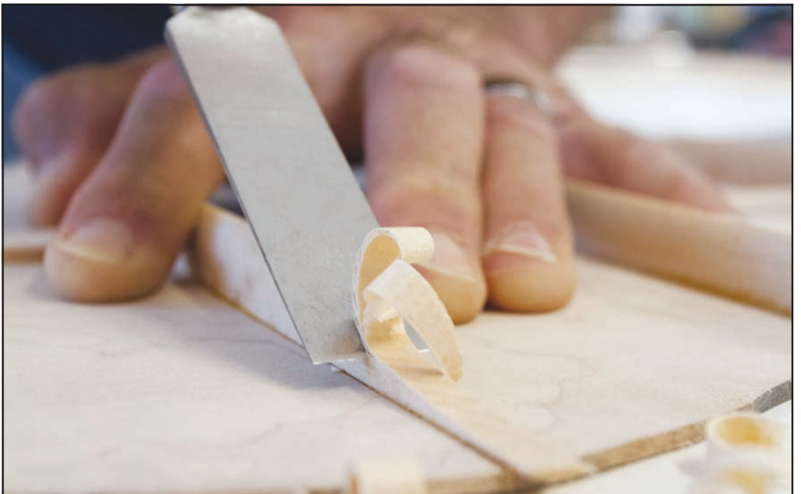
The bracing of Shawn Weimer's Zoe Guitars are hand carved. He avoids overbracing his guitars as that hinders the quality of sound the acoustic guitar may produce. Weimer said many brand name companies that mass produce acoustic guitars overbrace their guitars in an effort to prevent the instrument from breaking and being returned to the factory. That's the difference between a machine-built guitar and a handcrafted one.
