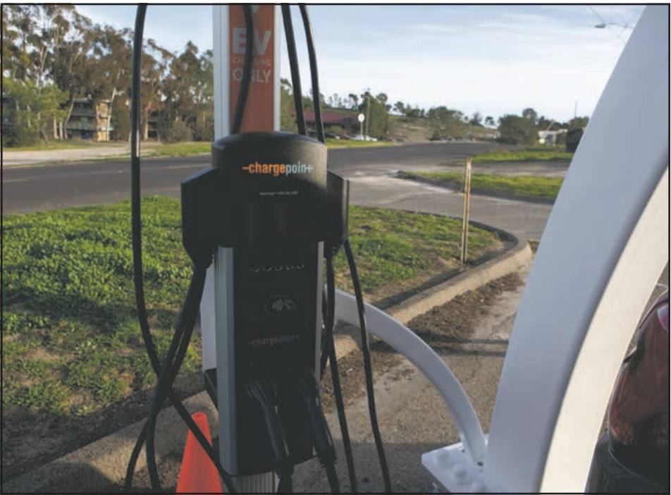
A Beam electric vehicle charger is being tested by Marine Corps Installations West's South West Region Fleet Transportation office in the 14 Area of Marine Corps Base Camp Pendleton, Jan. 12. Two of the new chargers, which operate independently from the power grid and can be used as batteries by first responders in emergency situations, will be tested on Camp Pendleton. U.S. Marine Corps photo by Lance Cpl. Shaina Jupiter
