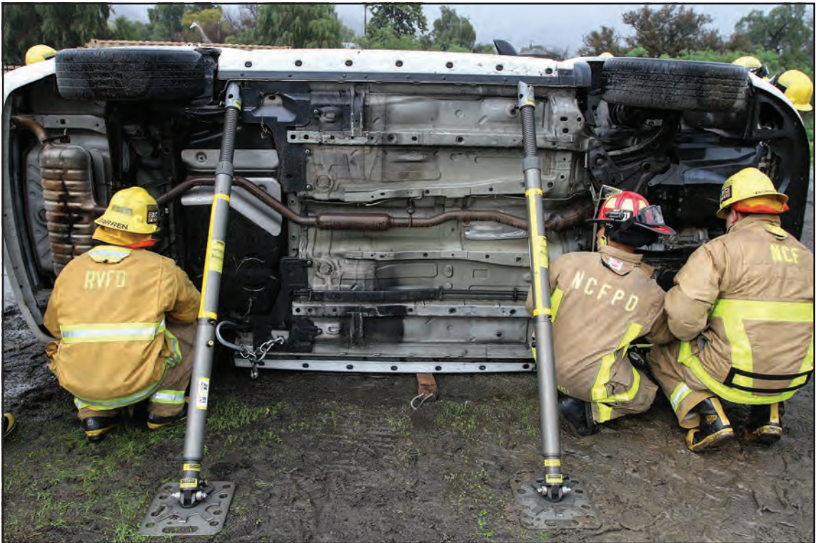
With the vehicle stabilization struts in place, North County Fire volunteers learn the remaining steps in further stabilizing a vehicle on its side.
