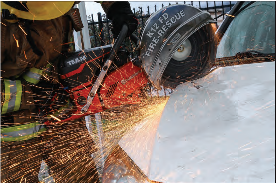
Volunteer firefighter students learn how to use a rescue rotary saw to cut into the hood of a crashed car.
