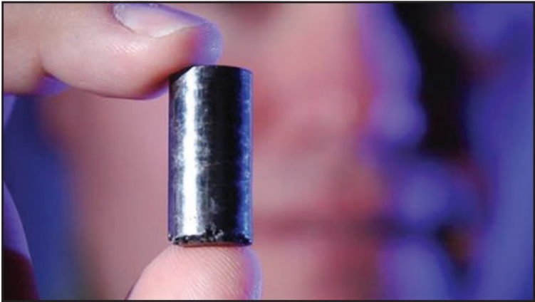
Ceramic uranium dioxide fuel pellets require 5,000 degrees Fahrenheit to melt.
